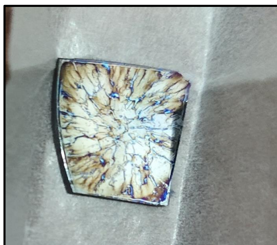
Fig.10 TiO 2 Deposited Substrate
