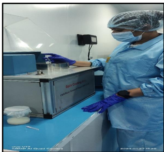
Fig.9 Deposition of TiO 2 on Si Substrate
